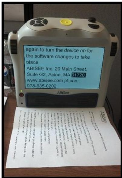
This simple document was aligned evenly in front of the device in landscape position with one side flush against the device. It scanned and read back with near perfect accuracy. The only error was that one period appeared as a comma on the print screen.
