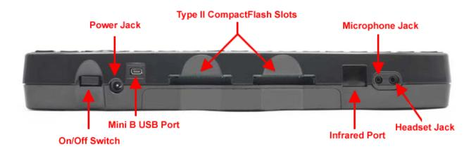
The CompactFlash slots on the BX400 support both CompactFlash Type I and Type II cards and peripherals. For a list of peripherals that have been tested and are recommended for the PAC Mate Omni, please visit http://www.PACMateGear.com.
