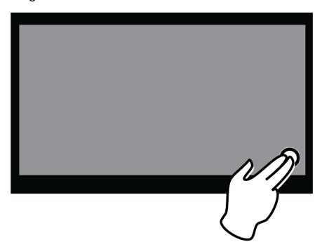
**Note:** To switch to OCR mode, the default method is to tap the screen in the lower right corner. This can be changed so that any tap on the screen while in video magnifier mode will automatically launch OCR mode. For more information, refer to **Activate Speech (Starting OCR Mode)** on page 55.
