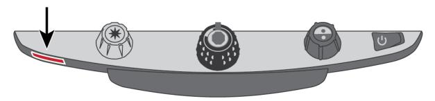
2. Press the button a second time to turn off Focus Lock, and restore automatic focus.
