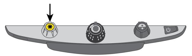
Crosshairs display on the screen (indicating the center of the image on the screen), and the camera zooms out.
