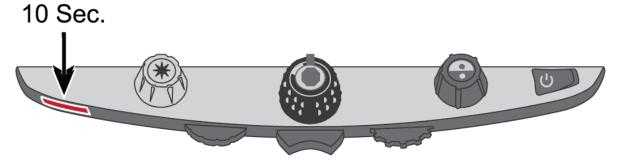
2. Press the **red Focus Lock button** until Freeze Frame **II** displays. It is selected (**√**) by default.
