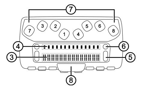
The refreshable braille cells (3) are located toward the front of the unit. There is a cursor router button (4) above each braille cell. At each end of the display's surface are NAV Rockers (5) used for easy navigation. Positioned above each NAV Rocker is a mode button (6) which cycles through the different navigation modes.
